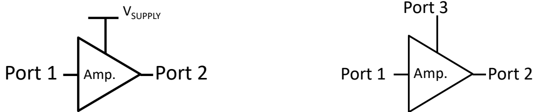
Figure 6. Amplifiers are traditionally treated as two-port circuits with a separate supply voltage (Left). Higher efficiency operation is accessed by treating the supply voltage as a separate independent input (right).
